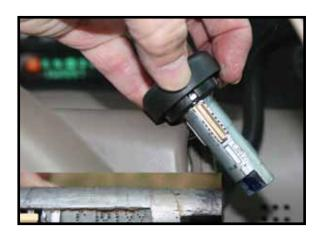
The process of determining the mechanical cuts is the same as with any other GM vehicle. If you are able to obtain the key code for the car, you will occasionally be able to get the resistor values as well – but don't count on it. If you are lucky enough to get the resistor value it will usually be given as a two character code which is also shown in sidebar two. On some of the later 10-cut ignitions, this resistor code is stamped onto the lock along with the code as shown.
